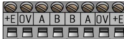
Picture 4 Terminal connections of power supply cables
